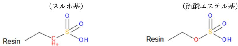
FIGURE 1 Difference between sulfonium-type (left) and sulfate-type ion exchanger (right)
